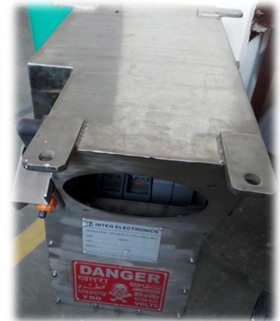
Feeder Junction Boxes are having working voltages up to 75 Volts and above 750 Volts. They contain polyamide conduits and accessories, terminal connectors, crimping sockets etc. as per the technical specification and drawing of Feeder Junction Boxes for respective railway coach.
